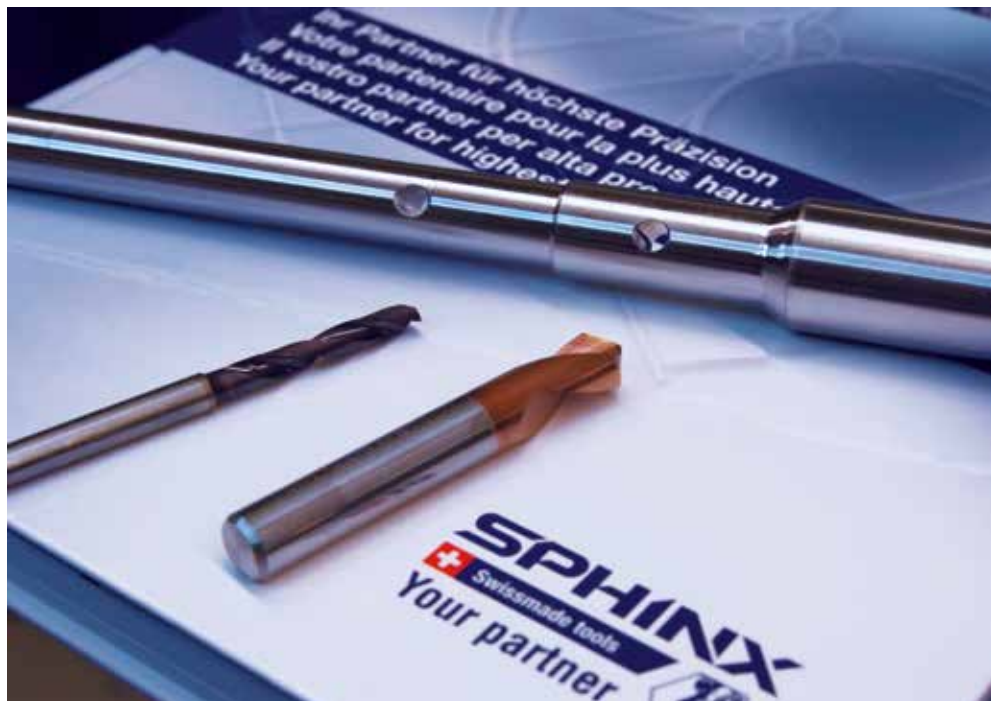
3 Radial drilling without centering: Optimum selection of technology parameters makes this possible using these high-performance drills (Photo: Mücke)
