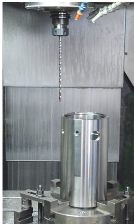
4 The solid carbide high-performance drills from Sphinx Werkzeuge enable reliable production on machining centres at a coolant pressure of just 20 bar
