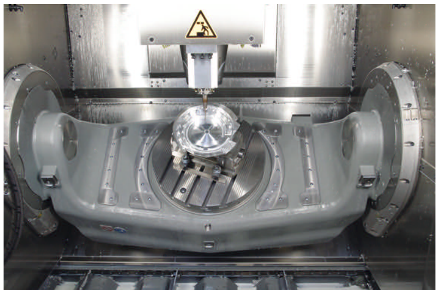
2 Completely in one chucking device: Five axes enable drilling and milling on five sides at any desired angle
